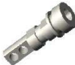
**SAFETY RELEASE VALVE** - The battery will operate above atmospheric pressure under normal operating conditions, however the maximum pressure is governed by the safety one-way release valve. Open is activated by pressures in excess of approx.(24-28 Kpa), resealing at approx.(8-16Kpa).
